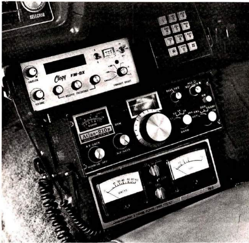
The Atlas transceiver fits nicely below the two-meter fm unit under the dash. The transceiver provides coverage of the amateur bands between 3.5 and 30 MHz. A power and SWR meter help to see that all is well with the transmitter and antenna system.
